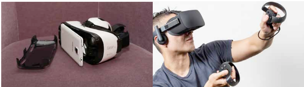
Gear VR with Galaxy Note 4 phone / Oculus Rift with Oculus Touch controllers
