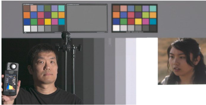
FIGURE 5: White balancing via the content's native color space provides the simplest way to balance wall content to a camera. This method may still introduce some, but less obvious particular color shifts in the image in comparison to simple RGB balancing within the display processing software. Example software interface courtesy of Blackmagic Design Pty, Ltd.
