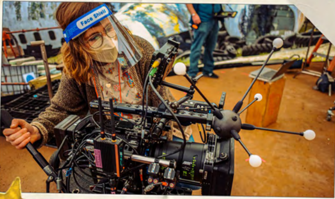
CINEMATOGRAPHER BOYD-BATSTONE IS SEEN HERE OPERATING THE ARRI ALEXA MINI LF FITTED WITH PASSIVE MARKERS. OPTITRACK CAMERAS LOCATED ALONG THE SEAMS WHERE THE LED WALLS MEET THE CEILING CAPTURE AND RELAY THE POSITION OF THE MARKERS WITHIN 3D SPACE TO A VIRTUAL CAMERA WITHIN UNREAL ENGINE THAT CONTROLS THE INNER FRUSTUM.
